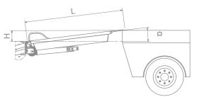
EXAMPLE: Let's assume we need to overcome a height difference (H) of 100 mm using an electric pallet truck. By applying the formula indicated above, we obtain: LENGTH OF BRIDGE OR TAIL LIFT IN 4% for manual pallet trucks, 8% for walk-behind electric pallet MILLIMETRES (L) = 100 mm x 100 / 8 = 1250 mm You must therefore select a bridge or tail lift with a minimum length of 1250 mm.
