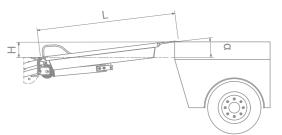
EXAMPLE: Let's assume we need to overcome a height difference (H) of 100 mm using an electric pallet truck. By applying the formula indicated above, we obtain: LENGTH OF BRIDGE OR TAIL LIFT IN 4% for manual pallet trucks, 8% for walk-behind electric pallet MILLIMETRES (L) = 100 mm x 100 / 8 = 1250 mm You must therefore select a bridge or tail lift with a minimum length of 1250 mm.
