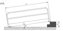
In case of adaptation, the aforementioned Italian regulation allows for steeper slopes in relation to the linear progression of the ramp. However, the ratio between slope and length must be of a lower value than what is shown by the interpolation line on the following graph (example: in case of adaptation, a maximum slope of 12% is permitted for lengths equal to or less than 3000 mm).
